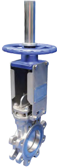
BKGV-A LUGGED ANSI 150 LB KNIFE GATE 316 Stainless Steel EPDM or Metal Seat 1000 KPA 50mm to 600mm
