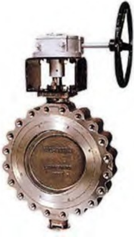
FSD CS (also STAINLESS NON FIRESAFE) HIGH PERFORMANCE BUTTERFLY VALVE PTFE Seat ASME B16.5 150 and 300 LB Firesafe Certified, Manual or Actuated -40 to 250 Deg C 80mm to 600mm 150lb 80mm to 450mm 300lb
