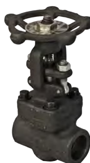
GL800 BB GLOBE VALVE API 602 A105N CLASS 800 (2000 PSI) Hard face seats Bolted bonnet 15mm to 50mm NPT Also available socket weld
