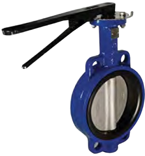
WEEL/WEEG CAST IRON BODY FBE Coated 316 SS Disc 410 SS Shaft EPDM Seat Gear or Lever operated 40mm to 300mm Rated 1600Kpa 350mm to 1200mm Rated 1000Kpa Suit AS2129 D/E and ASME B16.5
