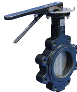
LANL/LANG CAST IRON BODY FBE Coated CFM8 SS Disc NBR Seat ISO Pad 410 SS Shaft Threaded Holes 50mm to 300mm rated 1600Kpa 350mm to 600mm rated 1000Kpa Suit ASME B16.5 Class 150 Only
