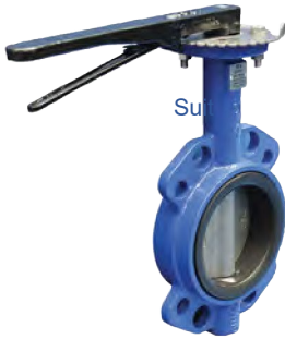
WEVL/WEVG CAST IRON BODY FBE Coated 316 SS Disc 410 SS Shaft Viton Seat Gear or Lever operated 50mm to 300mm Rated 1600Kpa 350mm to 600mm Rated 1000Kpa Suit AS2129 D/E and ASME B16.5
