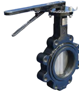
LAEL/LAEG CAST IRON BODY FBE Coated 316 SS Disc EPDM Seat 410 SS Shaft 50mm to 300mm rated 1600KPa 350mm to 600mm rated 1000Kpa Suit ASME B16.5 Class 150 Only
