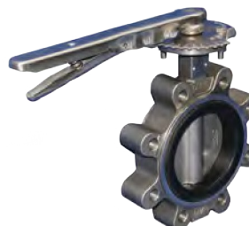
LEEL SS 316 BODY 316 Disc 316 SS Shaft EPDM Seat Gear or Lever operated 50mm to 300mm Rated 1600Kpa 350mm to 600mm Rated 1000Kpa Suit AS2129 E Only
