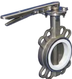
WETL/WETG SS 316 BODY 316 SS Shaft SS Disc PTFE Coated PTFE Seat Gear or Lever operated 50mm to 300mm Rated 1000Kpa Suit AS2129 D/E and ASME B16.5
