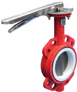
WETL/WETG CAST IRON BODY FBE Coated CI Disc PTFE Coated 316 SS Shaft PTFE Seat Gear or Lever operated 50mm to 300mm Rated 1000Kpa Suit AS2129 D/E and ASME B16.5
