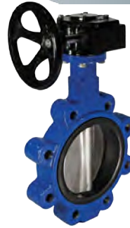
LEEL/LEEL CAST IRON BODY FBE Coated 316 SS Disc 410 SS Shaft EPDM Seat Gear or Lever operated 50mm to 300mm Rated 1600Kpa 350mm to 600mm Rated 1000Kpa Suit AS2129 E Only
