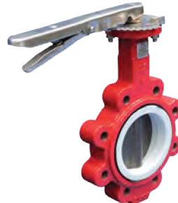
LETL/LETG CAST IRON BODY FBE Coated CI Disc PTFE Coated 316 SS Shaft PTFE Seat Gear or Lever Operated 50mm to 300mm Rated 1000Kpa Suit AS2129 E Only
