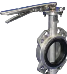
WEELSS 316 BODY 316 Disc 316 SS Shaft EPDM Seat Gear or Lever operated 50mm to 300mm Rated 1600Kpa 350mm to 600mm Rated 1000Kpa Suit AS2129 D/E and ASME B16.5
