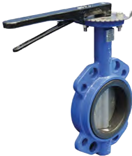
WENL/WENG CAST IRON BODY FBE Coated 316 SS Disc 410 SS Shaft NBR Seat Gear or Lever operated 50mm to 300mm Rated 1600Kpa 350mm to 600mm Rated 1000Kpa Suit AS2129 D/E and ASME B16.5
