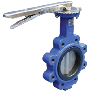
WEVL/WEVG CAST IRON BODY FBE Coated 316 SS Disc 410 SS Shaft Viton Seat Gear or Lever operated 50mm to 300mm Rated 1600Kpa 350mm to 600mm Rated 1000Kpa Suit AS2129 D/E and ASME B16.5
