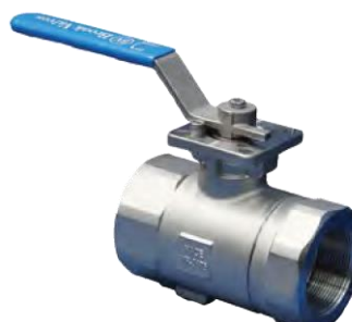
V2 2 PIECE BALL VALVE 316 Stainless Steel Full Bore Lockable Lever PTFE Seats 8mm to 100mm BSP Also available with NPT thread 1000 PSI
