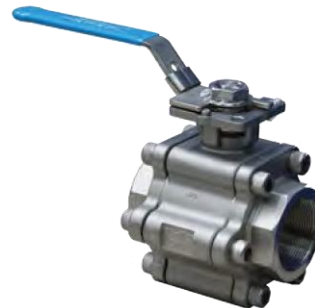
V3FSFB/RB 3 PIECE BALL VALVE Firesafe Certified, ISO PAD Lockable Lever Operated 316 Stainless Steel Full Bore / Reduced Bore PTFE Seats 8mm to 50mm NPT 2000PSI
