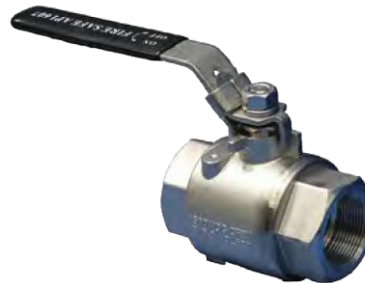
V2DM 2 PIECE BALL VALVE 316 Stainless Steel Reduced Bore PTFE Seats 8mm to 50mm NPT 2000 PSI 8mm to 15mm Full Bore
