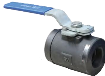
BL1500 BALL VALVE NPT CLASS 1500 (3700PSI) A105N 2PCE CTFE SEATS Firesafe Certified, Full Bore Lever Operated 15mm to 50mm
