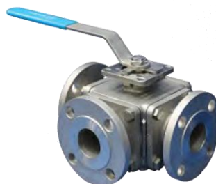
3WAYL/3WAYT-ISO-150 3 WAY FLANGED ANSI 150 BALL VALVE 316 Stainless Steel TMF 1600 seats ISO Mount Full Bore L or T Port 25mm to 250mm
